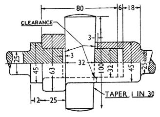
SOCKET AND SPIGOT JOINT Figure No. 2
